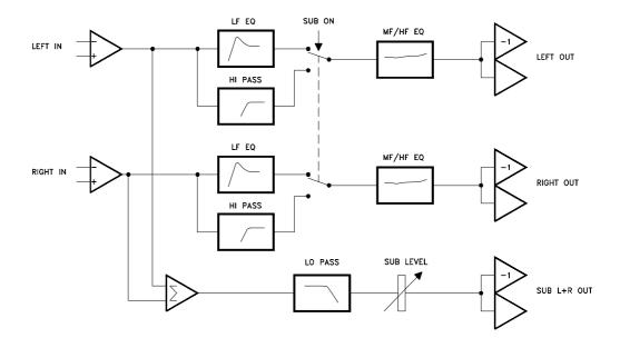
Figure 4. TX2 simplified block diagram.
